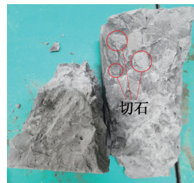
图6 高强度组 60%含石量试样破坏面 Fig. 6 Failure surface of 60% block content samples in high strength group
